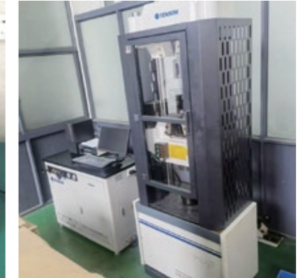
▲ Universal Testing Machine Testing the tensile force of bolts and the load - retaining capacity of nuts
