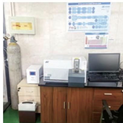
▲ Spectrometer Testing the chemical composition of materials
