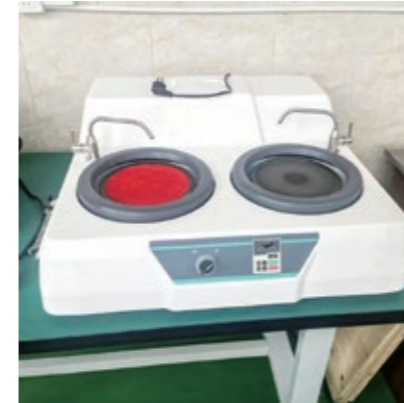
▲ Grinding and Polishing Machine Pre - grinding and polishing
